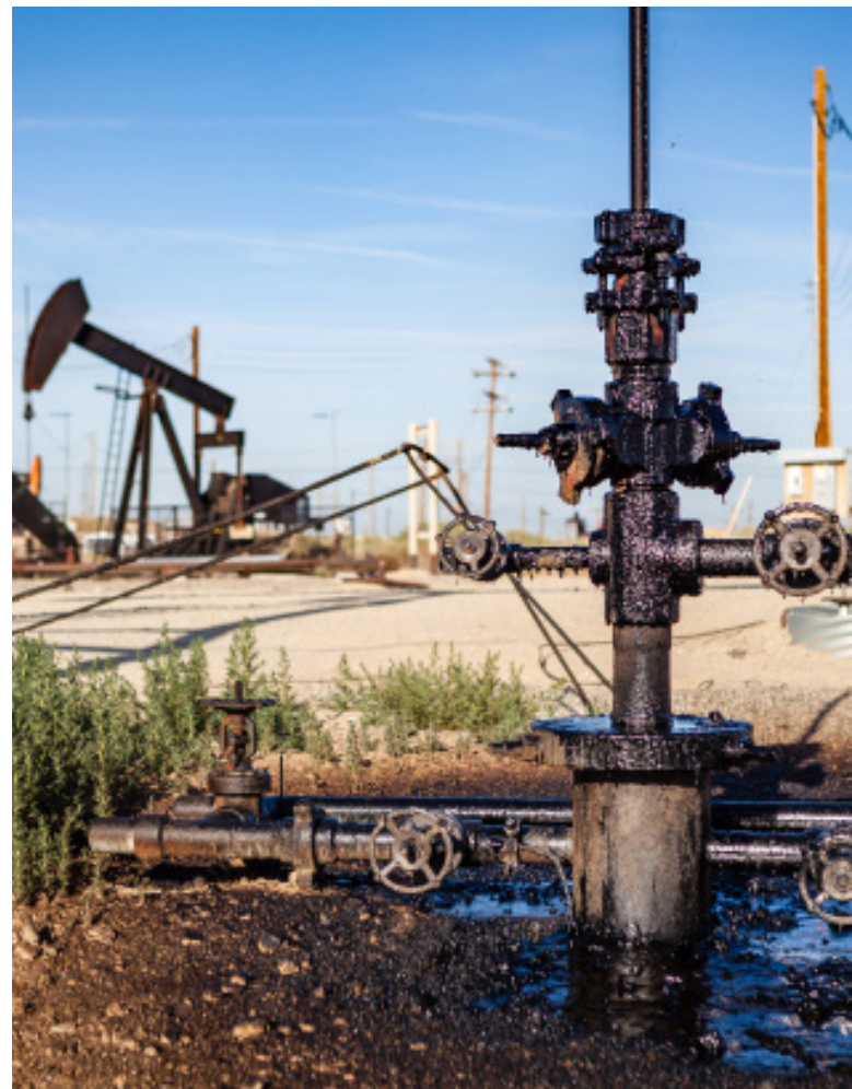
AN OIL PUMPJACK WITH A LEAKY WELLHEAD DRIPS OIL ALONG THE SIDE OF THE ROAD IN CALIFORNIA © GARY KAVANAGH VIA ISTOCK
