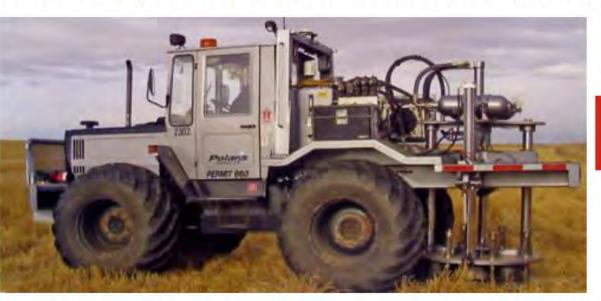
Polaris 860 Seismic Tractor : Lightest impact equipment available
